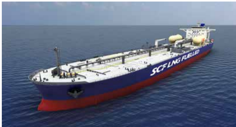
The amount of gas on board SCF's LNG fuelled Aframax is about 1,700 cubic metres according to current specifications. This is enough for a cruising range of 21 days with operation on gas at full speed.
