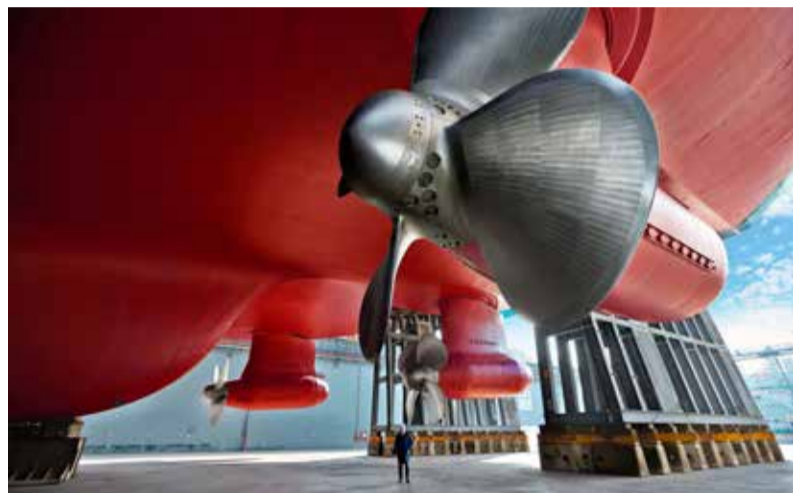
The propulsion system of the new gas carrier consists of three Azipod-type propulsion units.
